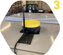
Install FieldBee controller on the tractor's roof
